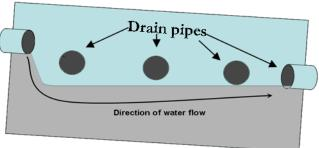
An unlevel distribution box forces all of the septic wastewater into 1 drain line. This causes the water to appear above ground because the soil is saturated.
