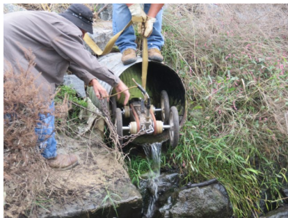
Above left: Video inspections of spillway pipes Above right: embankment regarding on flood control dams
